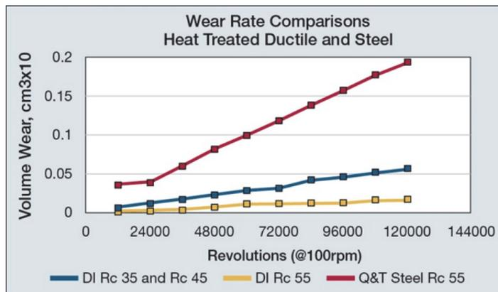
Data is based on 3 pad specimens on 52100 hardened steel disks, dry conditions, 150 lbs. force.
