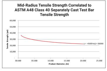
Continuous cast bars made from Dura-Bar G2 can be certified to ASTM A48, class 40 when the separate cast test coupon has a minimum tensile strength of 40,000 psi. As mentioned previously, separate cast test bar tensile strengths will be much higher when poured from iron used to produce 20.0" diameter continuous cast bars than with iron used to make 2.0" diameter bars.
