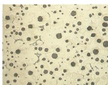
60-40-18 contains nodular graphite in a matrix of all ferrite and is the softest ductile iron grade. There is very little difference in machinability between this grade and 65-45-12, and it is rarely used because of the added cost of heat-treating.
