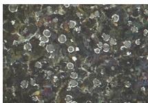
100-70-03 is highly pearlitic with only small amounts of ferrite. This grade has the best wear resistance of the as-cast ductile irons and is used in applications requiring good strength and high wear resistance. It is also the least machinable grade and normally used as an alternative to heat-treated steels requiring hardness values below 302BHN.
