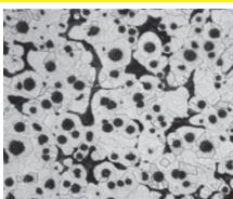
65-45-12 has a ferritic matrix structure with small amounts of pearlite and is very similar to low-carbon steel grades. In bar form, it is an excellent replacement for low-carbon leaded steels as well as rephosporized and resulfurized free machining grades including:
