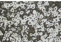
80-55-06 contains approximately 50% ferrite/50% pearlite, although the composition can vary depending on the producer. This grade is slightly less machinable than 65-45-12 and is used when better wear resistance and higher strengths are required. It is a good replacement for medium carbon steels including:
