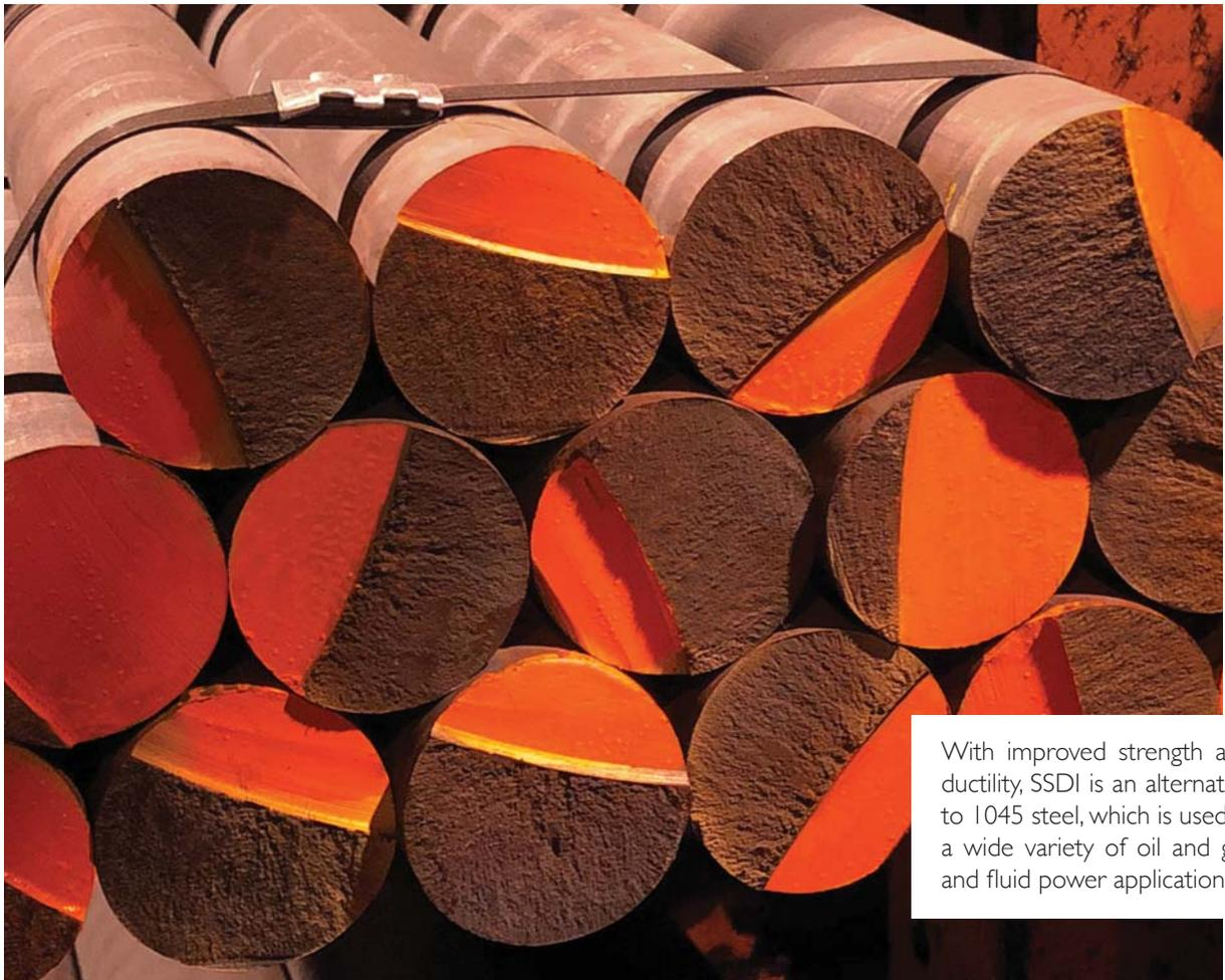
With improved strength and ductility, SSDI is an alternative to 1045 steel, which is used in a wide variety of oil and gas and fluid power applications.
